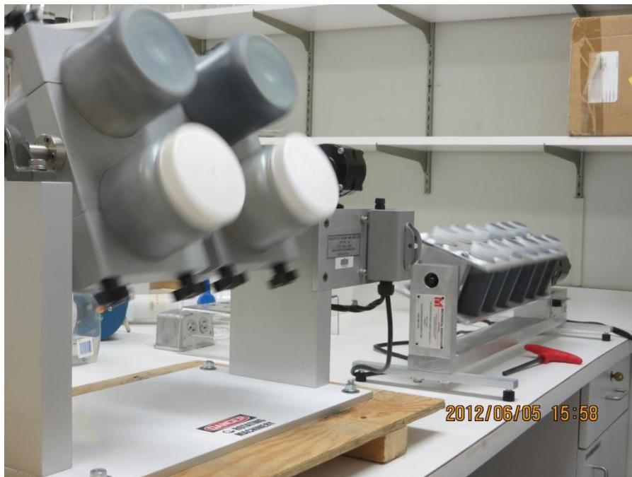
Figure 3 Rotary agitators tumbling samples for Method 1313 and Method 1316
