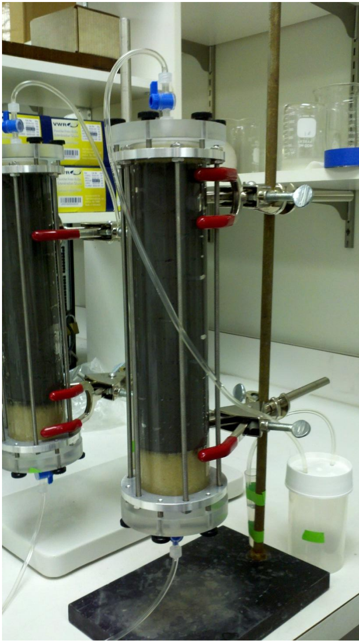
Figure 2 up flow columns ready for liquid to solid ratio material testing
