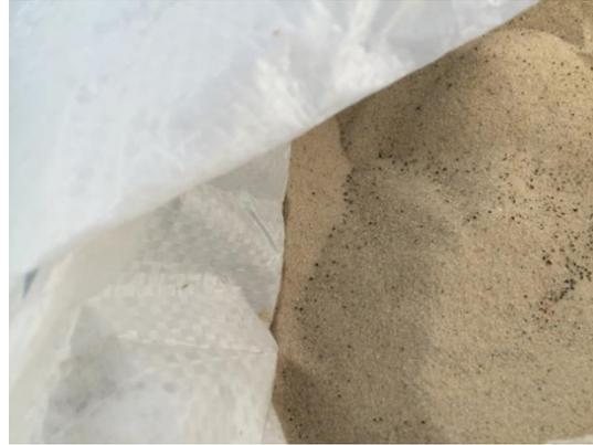
**Figure 8: Typical jetted wellpoint materials – geotextile screen and a properly graded sand maximizes yield**
