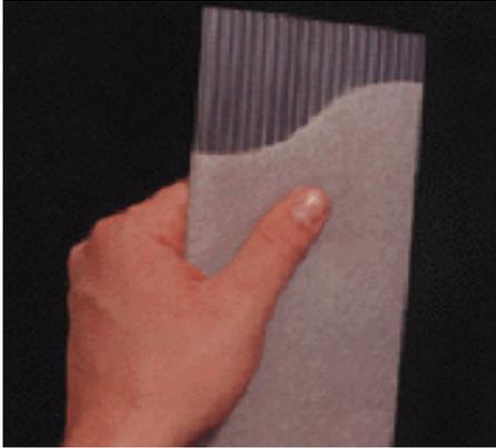
**Figure 7: A non-woven wellpoint geotextile fabric will restrict the flow of water**
