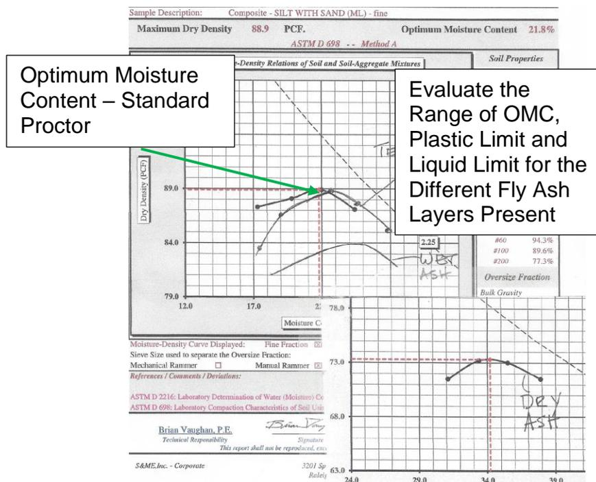
**Figure 4: Typical Field Curve for Moisture Content Evaluation**
