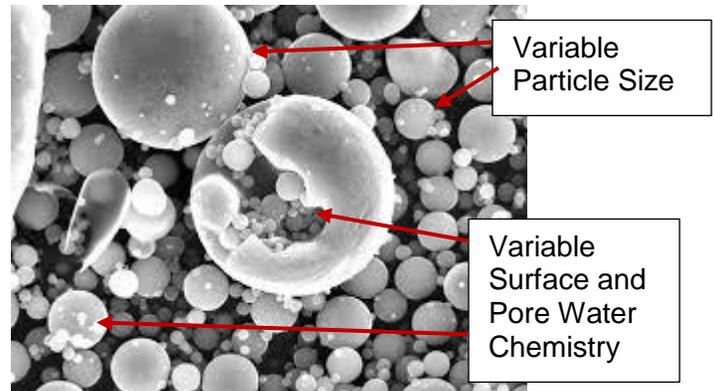
**Figure 3: Typical Fly Ash in Ash Basins**
