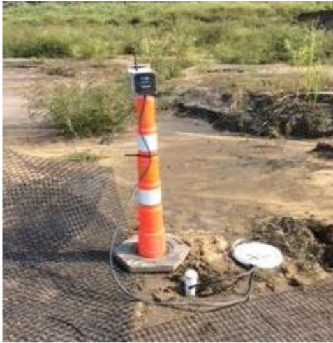
**Figure 5: Typical “real-time” pore water pressure reading device**
