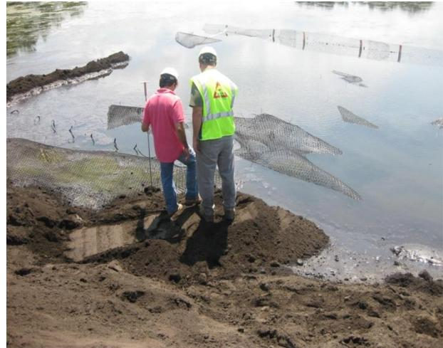
**Figure 6: Hand held vane shear test readings safely obtained over geogrid**
