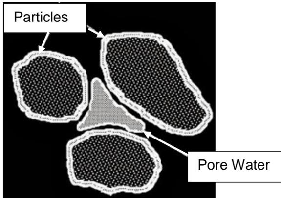
**Figure 2: Soil Moisture Diagram**
