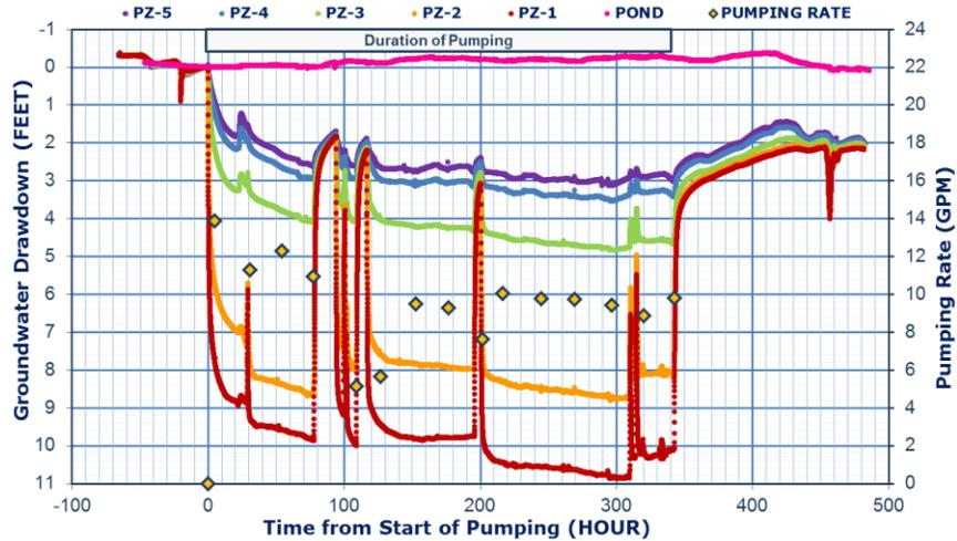
**Figure 1: Typical Pump Test Curve**
