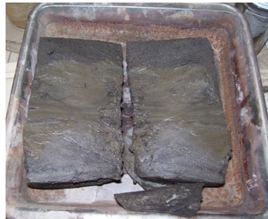
Figure 2: Sample of Layered Ash Basin Less Drainable and More Drainable Ash
